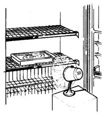
4. Place pans of hot water inside freezer to hasten melting of frost. Leave door open. As ice softens and melts, it can be removed in large pieces. Direct air from an electric fan into the freezer to speed defrosting.
